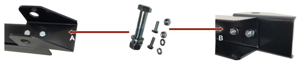
TOP VIEW: Use the 2) 1/4" x 3/4" bolts and insert them thru both holes with the receiver mount base
