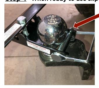
To mount your Garbage Hook to your receiver hitch simply insert the 3/8" retainer pin thru the ball mounting base and under your 1-7/8" or 2" ball. 2" Ball works best
