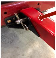
SR-MT receiver base slips unto the two upright flanges of the installed BRH and pined in place.
